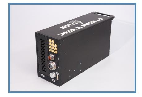
"Our new extremely rugged ½ ATR recorder provides real-time sustained recording rates up to 4 GB/s," said Chris Tojeira, Recording Systems director, Pentek. He added, "We can capture the full bandwidth of all eight 250 MHz 16-bit phase-coherent A/Ds in this single compact chassis."
